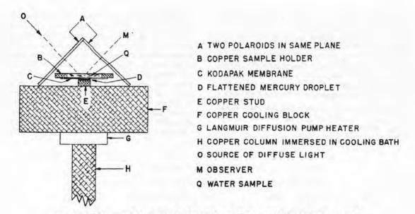
APPARATUS USED FOR FREEZING EXPERIMENTS WITH WATER
